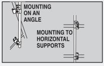
Flexible Clamps allow installation at any angle.
