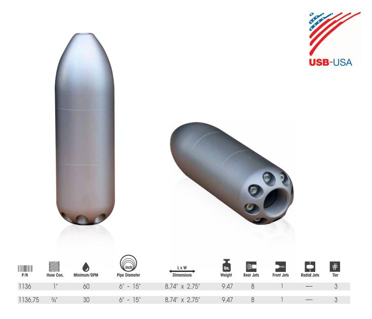
**Used in pipes that may have holes in the bottom or offsets**, the 3D Extreme nozzle is a worthy tool to have in your tool box, 3D fluid mechanics inside of the nozzle and one-piece ceramic inserts create a strong jet pattern with a spray angle of 11° resulting in exceptional cleaning and pulling power. One forward jet offers a penetration option as well.
