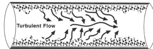
Choked Down Pipe
