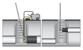
**ALWAYS BLOCK PLUGS WHEN CONDUCTING AIR TESTS.**
