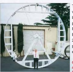
This joint tester was designed and built for a water project near Phoenix, Arizona. Each joint of this 21' diameter pipeline was tested at 30 PSI.
