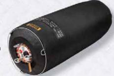
The second patent covers our superior end design. The ends are reinforced with a steel "spider™" ring wrapped in fabric. The fabric extends from the spider™ into the body of the plug. This advanced design transfers the stress of the inflation through the fabric to the steel spider™ ring leaving the bond at the base plate at a more relaxed state.
