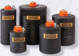
The SST™ and MST™ Plugs are designed with multi-function in mind. Available in single sizes 8" through 24" and multi-size 8"- 12". Each of these have a 3" female NPT aluminum by-pass. These plugs can be used to stop flow, for sewer by-passing, or for air testing. An air test conversion cap comes supplied with every SST™ and MST™ Plug.
